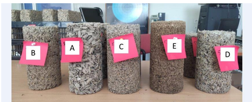
Figure 6. The concrete cylindrical samples with a 1:3 ratio of wood particles to cement, produced by Institut Technologique FCBA.
