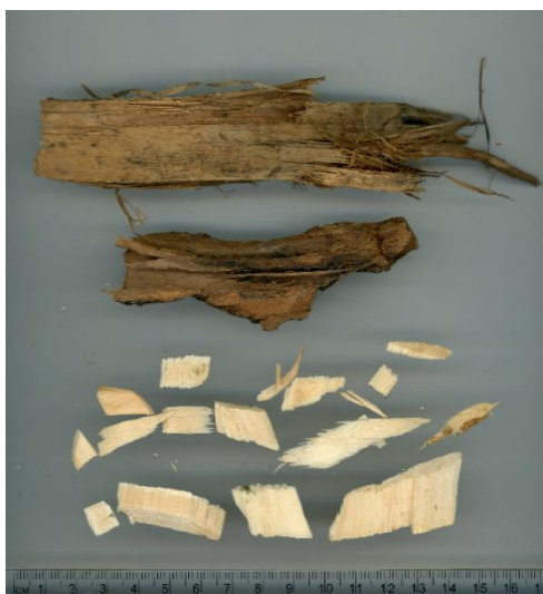
Fig 2.5. Parts of the samples analyzed (bark and wood) for characterization of pH, pH buffer, ash levels and ICP analysis of contaminants of reference poplar.
