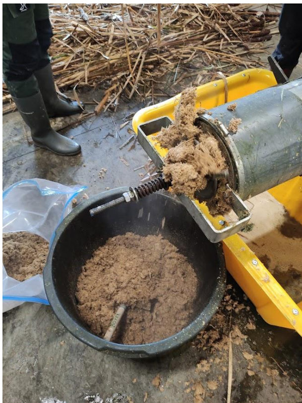
Figure 3: Extruder being used on autumn biomass in Grassa biorefinery. Field extrusion would remove 34% of the moisture from the fresh weight substantially reducing the transportation and drying costs. Photo: Sannimari Käärmelahti.
