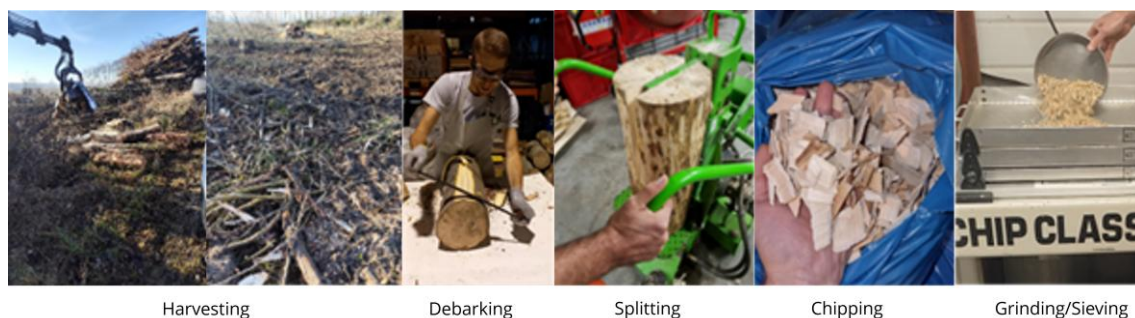
Figure 15. Processing steps for wood: harvesting, debarking, splitting, chipping into wood chips, grinding into particles, and screening. Photos: Edern Philippot.
