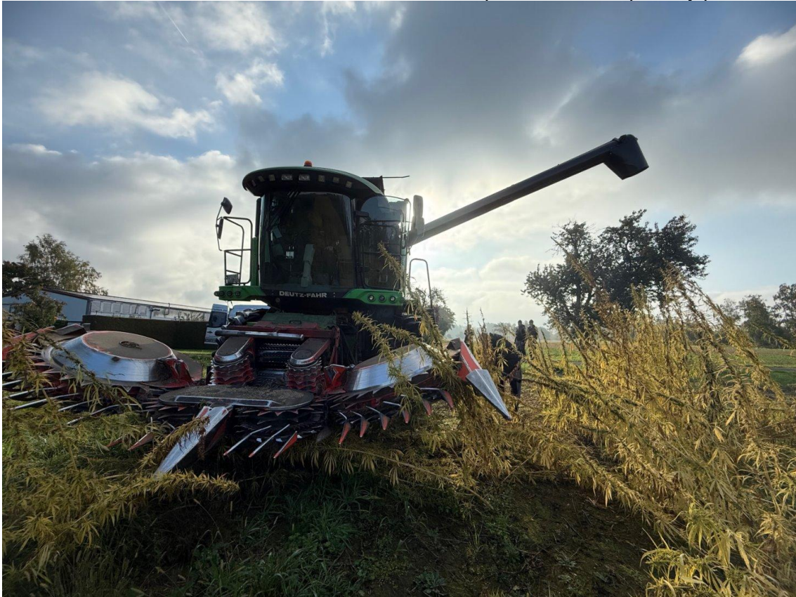
Figure 12. Industrial hemp harvest in Bühl with a combine harvester equipped with a modified Kemper corn deep-cut cutting unit. Photo: Almut Frank.
