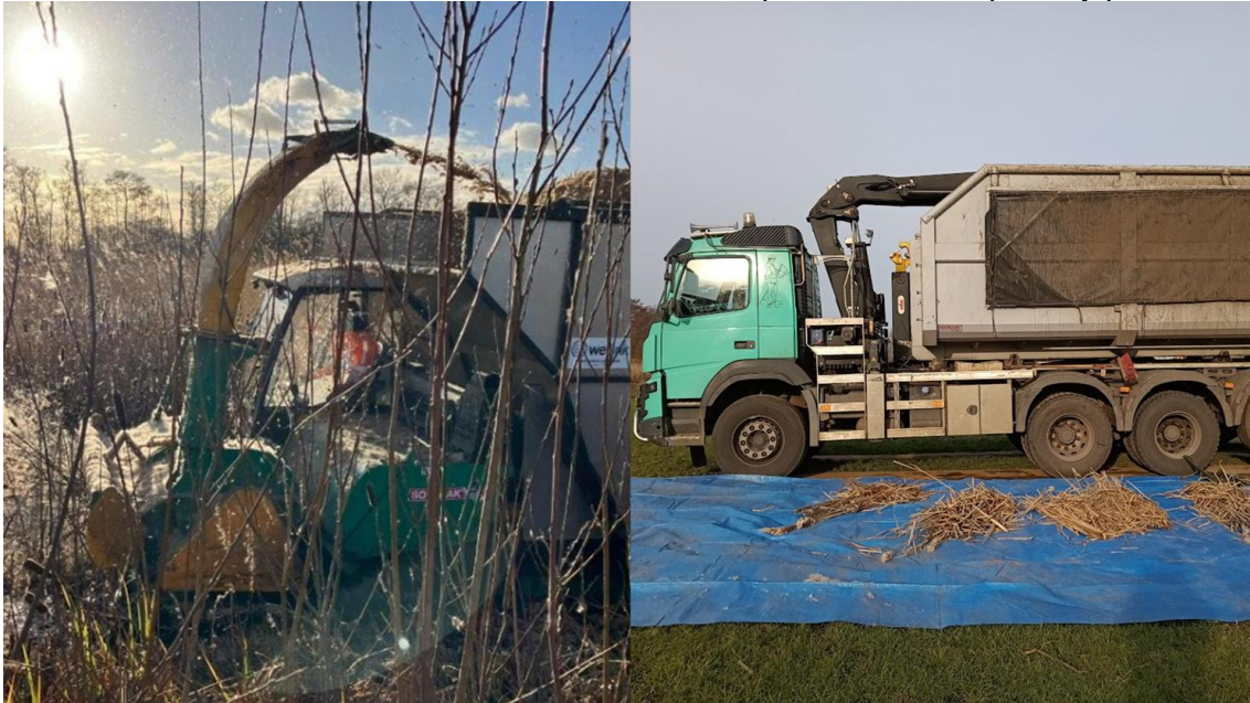
Figure 1: Typha harvester (Loglogic wetland mower, left) and a tipper truck (right) in Ankeveen pilot site. In this scenario, biomass is directly transported without volume reduction from the field to a drying facility. Photos: Christian Fritz (left) and Sannimari Käärmelahti (right).
